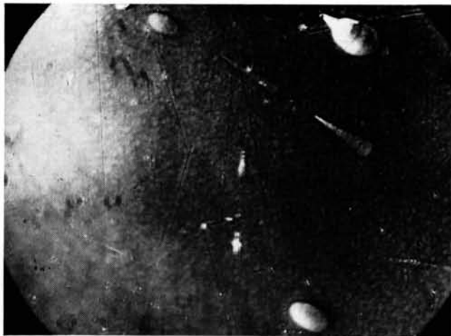
Fig. 1. 'Tadpoles' and elliptical features on cultured quartz ( \times 56 ).
