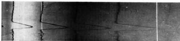
Fig. 3. Fringes of equal chromatic order proving the 'tadpoles' to be elevations.
